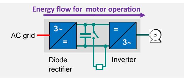
In **braking** mode, the inverter needs to dispose of the stored energy.
